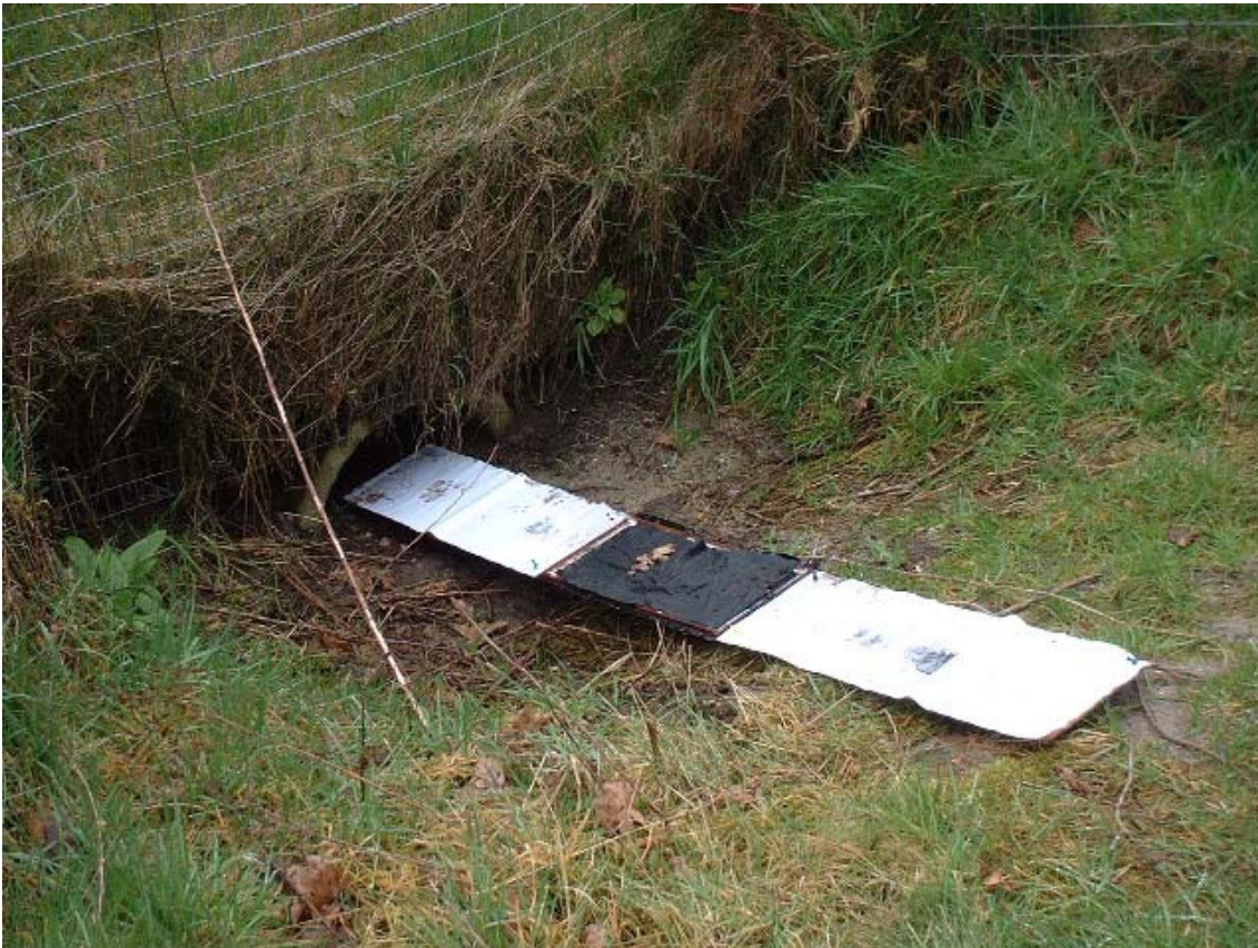
Figure 1. Track board with inking pad and paper sheets at the entrance of a fauna pipe.
